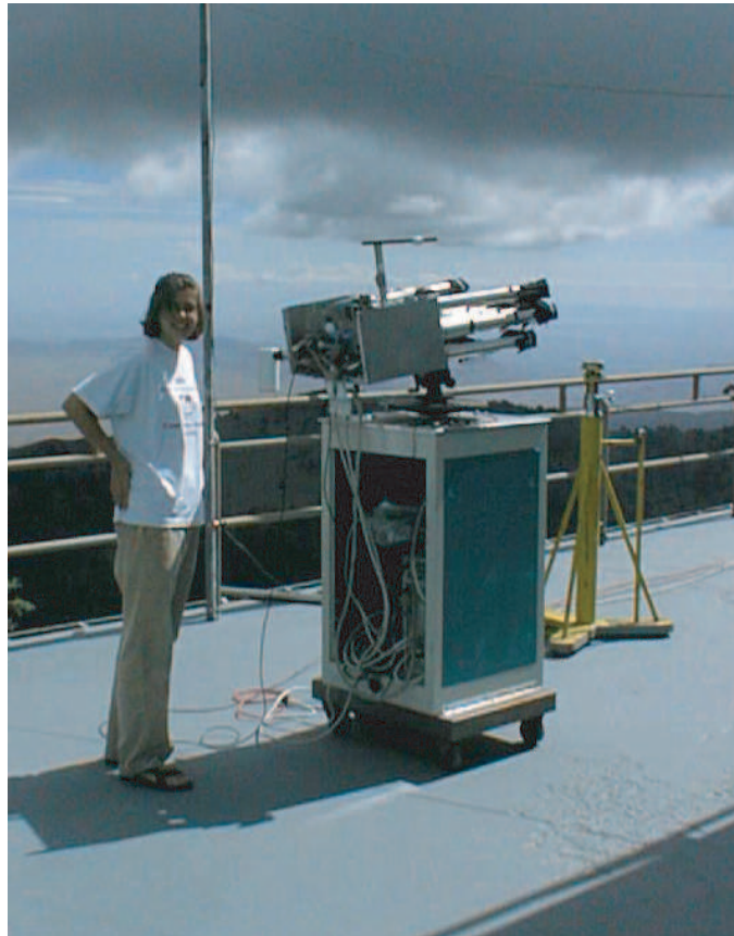
Figure 3-9: The Fly’s Eye deployed at Langmuir Laboratory. The Fly’s Eye (shown here with the video system removed and with fellow student Elizabeth Gerken) is mounted on a rack which contains power supplies and the control/data acquisition computer. The video recorders and the GPS receiver are located inside the laboratory.
